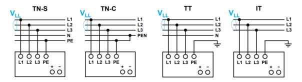
Fig. 4 AC Input Operation Connection Diagram
