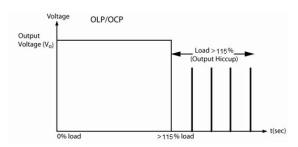
Additionally, if the  $I_0$  is < 115% but > 100% for a prolong period of time (depending on the load), the Over Temperature Protection (OTP) will be activated due to high temperature on critical components. The power supply will then go into "Hiccup mode" until power supply cool down.
