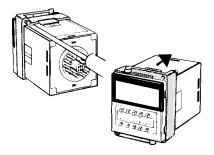
Several timers may be mounted close together using Y92F-30 adapter as shown here. When mounting two or more timers in a vertical line, arrange the adapters so that their molded tabs are positioned on the right and left sides. When mounting two or more timers in a horizontal line, arrange the adapters so that their molded tabs are positioned on the top and bottom sides.
