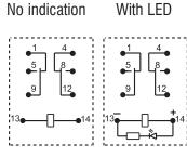
Remark: For AC parts with diode, the positive and negative pole markings on wiring diagram are not applicable.
